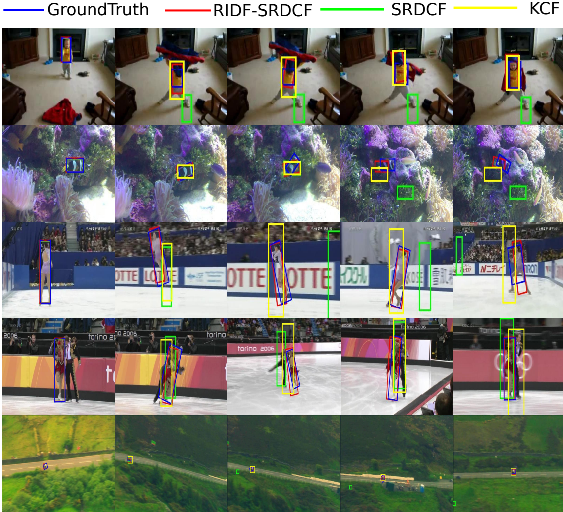
Figure 5.6: Qualitative analysis of RIDF-SRDCF compared with baseline SRDCF and few other correlation filter trackers. The proposed tracker performs favourably against the other correlation filter trackers. The rotation adaptive filters assist in determining the orientation of the target object effectively that leads to substantial gain in overall performance.
