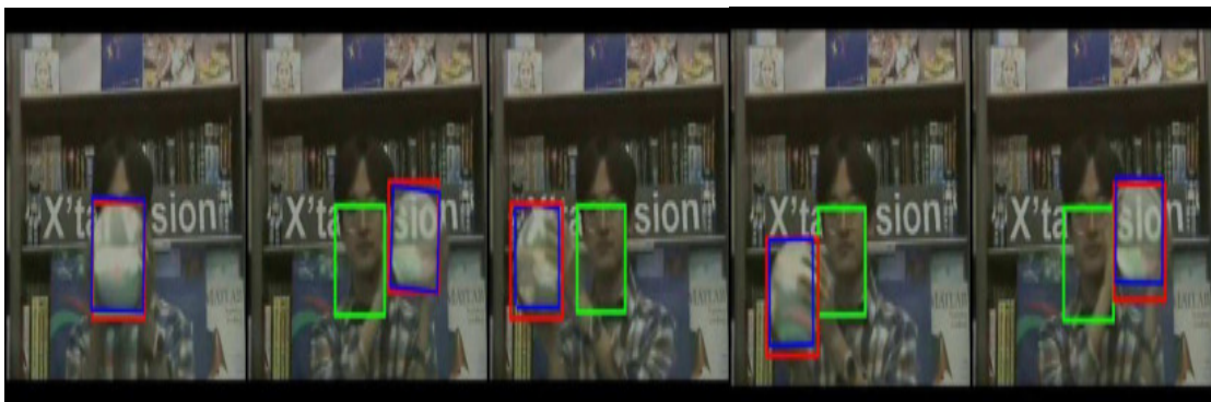
Figure 3.10: Sample frames from the sequence sphere of VOT2016 [5]. The blue, green, and red rectangle shows the groundtruth, SRDCF, and I-SRDCF (with IC) outputs, respectively.
